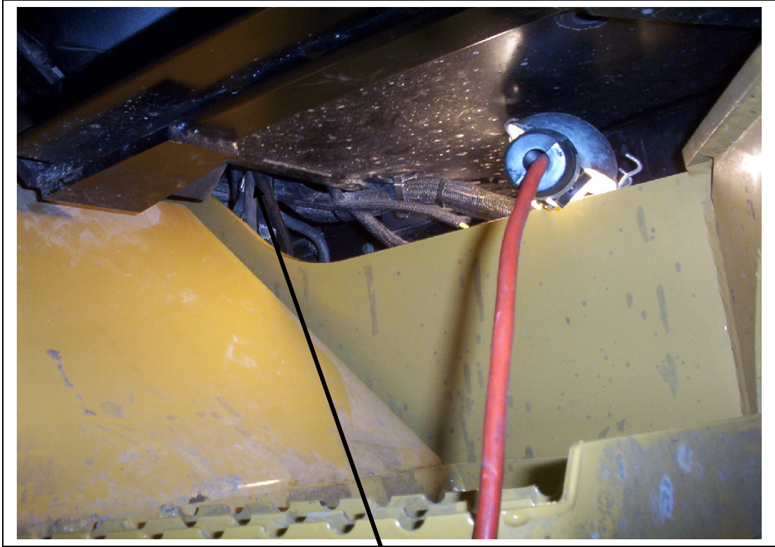
Clutch wire and thermostat probe under the cab.
