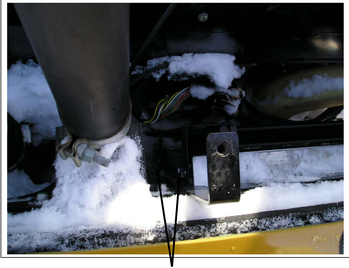
Mounting nuts on the left end of the condenser coil.
