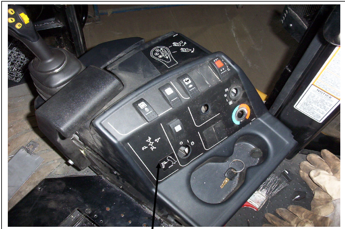
Thermostat and decal in place in right hand control console.
